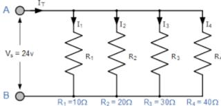
(iv)Identify the type of combination of resistors from the following figure
